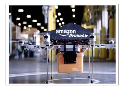
The drone used by Amazon Prime Air is an octocopter, meaning that it has eight rotor blades arranged in an octagonal manner.
